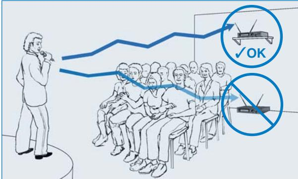
proper and improper antenna and receiver placement
