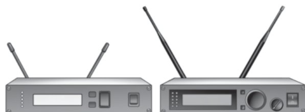
Figure 2-27: 1/4 wave and 1/2 wave antennas UHF range
