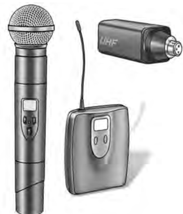
Figure 2-2: examples of transmitters (left to right: handheld, bodypack, plug-on)
